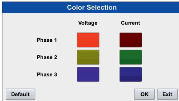
User can select particular color for each phase from some fixed defined colors by clicking on the phase color tab on previous screen. It displays the old and new color also.
