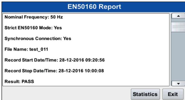
The screen shows whether synchronous connection is present or not. If not then it is in Islanded Mode. It also displays start time and stop time of recording. If all parameters are within specified range then result shown is Pass.
