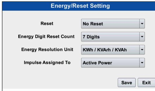
The screenshot shows a configuration window titled "Energy/Reset Setting". It contains four rows of settings, each with a label on the left and a dropdown menu on the right. The settings are: "Reset" set to "No Reset", "Energy Digit Reset Count" set to "7 Digits", "Energy Resolution Unit" set to "KWh / KVAh / KVAh", and "Impulse Assigned To" set to "Active Power". At the bottom right of the window are two buttons labeled "Save" and "Exit".
