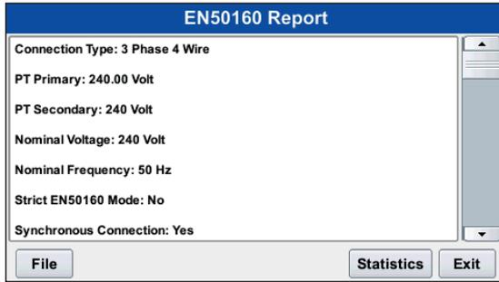
The above screen displays the basic settings of meter such as connection type, PT primary, PT secondary, nominal voltage, nominal frequency and whether strict compliance mode of EN50160 is enabled or not.
