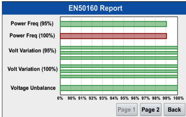
In above figure, the red color of power frequency indicates that frequency is below preset limits for required % of time. Hence result of frequency is fail. Green color of supply voltage unbalance indicates that the voltage unbalance is within preset limits for required % of time and hence result is pass for that particular parameter.
