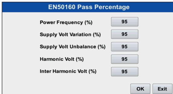
The EN50160 Pass Percentage screen features a blue header with the title "EN50160 Pass Percentage". Below the header, there are five rows, each with a parameter name and a value in a button: "Power Frequency (%)" with value "95", "Supply Volt Variation (%)" with value "95", "Supply Volt Unbalance (%)" with value "95", "Harmonic Volt (%)" with value "95", and "Inter Harmonic Volt (%)" with value "95". At the bottom right, there are two buttons: "OK" and "Exit".
